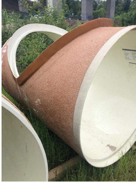
Figure 1 - GRP Liner - Note the bonded brown aggregate outside and smooth inside
